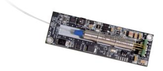
DiCon's PM MEMS 1xN Optical Switch provides channel selection between a single input fiber and N output fibers. At the core of the switch is DiCon's proprietary MEMS chip; an electrostatically driven mirror implemented using single-crystalline silicon and a stiction-free design. The mirror is capable of rotating on two axes, allowing the input light to be redirected back to any desired output. The switch is bi-directional and can be used as a Nx1 selector switch.
