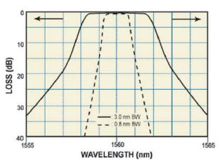
NOTE: Optical Spectrum example above is for the C Band option \*The L Band option has a similar 0.8 nm BW shape
